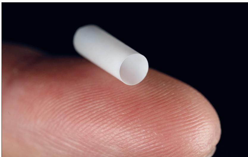
Fig. 1 Miniaturised and resistant ceramic sleeve made of Rapal® 1000 ZA
